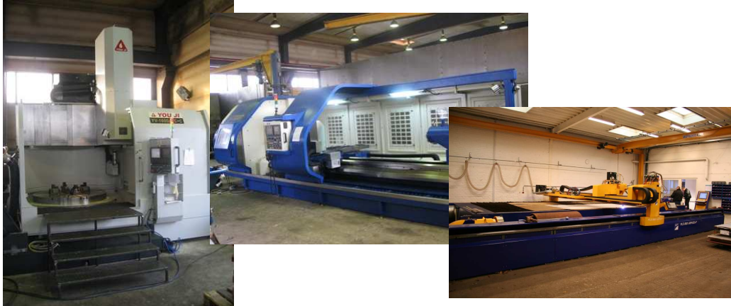
Left: CNC Vertical Turning Lathe with a work-piece capacity of \varnothing 2.000 \times height 1.200 mm Middle: CNC Horizontal Turning Lathe with a work-piece capacity of \varnothing 1.010 \times length 4.000 mm Right: Cutting center with table area 8.000x3.000 mm – Plasma 3-40 mm in stainless and mild steel – Cutting burner up to 140 mm in mild steel
